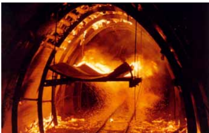
Fig. 5. Testing a conveyor belt in the DMT fire testing gallery to determine its suitability for use underground in accordance with DIN EN 12881-2.
