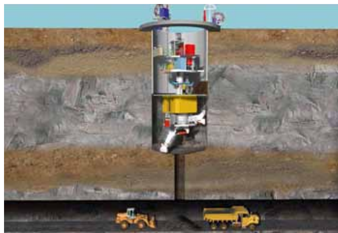
Fig. 1. Shaft sinking with a shaft milling machine.
