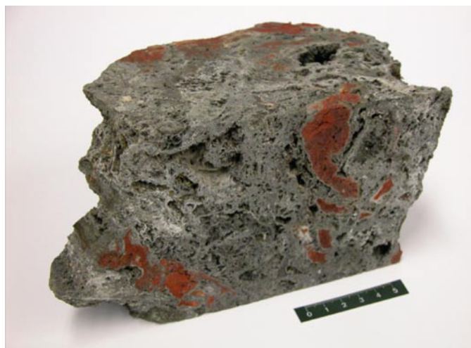
Fig. 4. Massive sulphide sample with high copper content, taken from the Indian Ocean.
