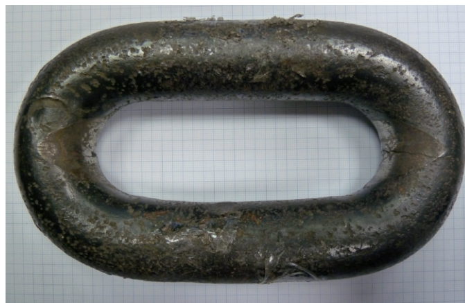
Fig. 6. Pitting and crevice corrosion on a chain link.
