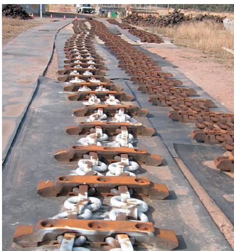
Fig. 5. Chain assembly undergoing examination for corrosion damage above ground.
