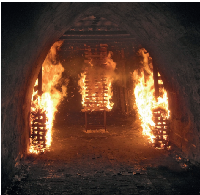
Fig. 6. Real scale test for cavity filling foams with a 460 kg wood fire object shortly after ignition.
