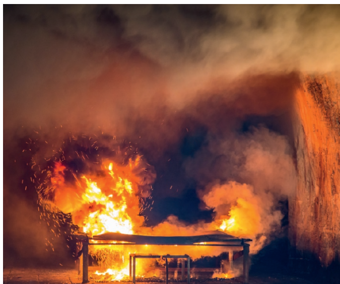
Fig. 3. DIN EN 12881-1, method A shows the test of a conveyor belt which does not fulfill fire safety requirements. Spreading of flames to the belt and smoke must be noted.
