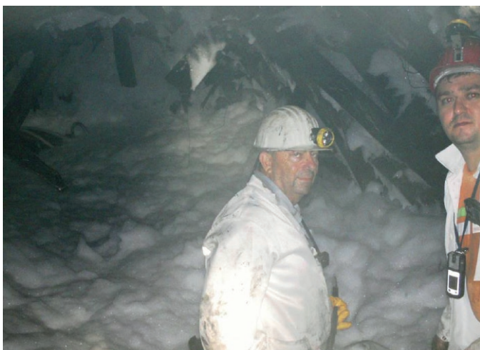
Fig. 12. Result of foam discharging: The Kalın Damar headgate is totally inundated with foam.
