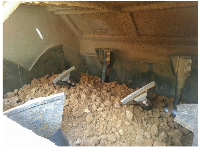
Fig. 6. Material mixed with quicklime during the mixing process in the Combimix system at CEMEX France.
