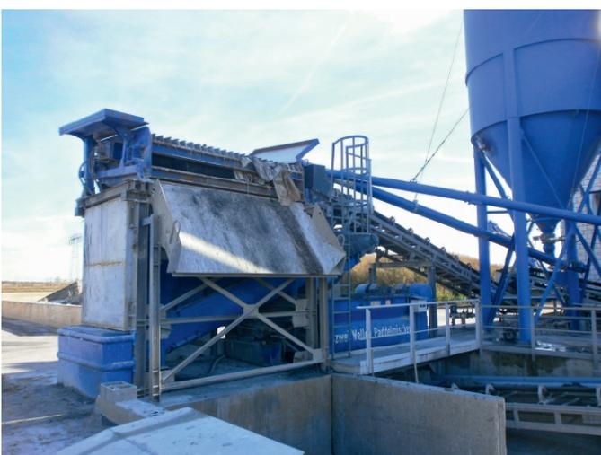
*Fig. 3. A twin-shaft continuous mixer of type LFKR 1130 stabilizes sludges with mineral matter, fly ash and water, enabling the product to be disposed of.*
