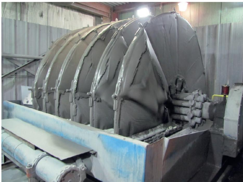
*Fig. 1. SA disk filter reduces the high quantity of water in the suspension, which is yielded when processing gold ore in one of the world's largest gold mines.*
