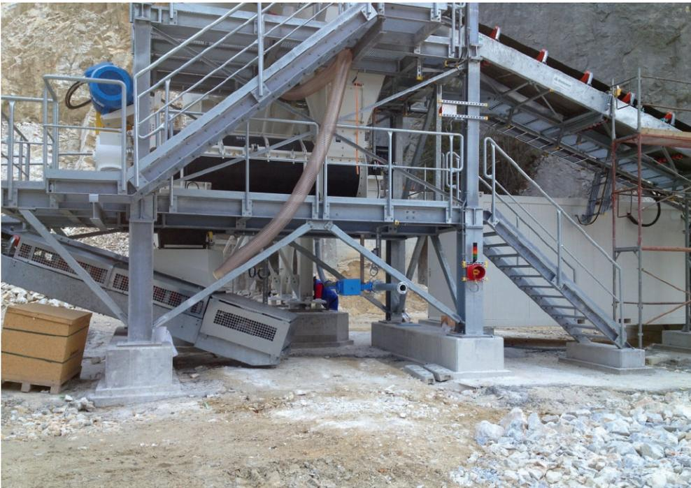
*Fig. 2. A single-shaft continuous mixer of type MFKG 1032 conditions up to 450 t/h of flotation tailings. This will allow the weatherproof mixed material to be disposed of in an abandoned section of the mine in a manner that prevents leaching of the harmful substances.*
