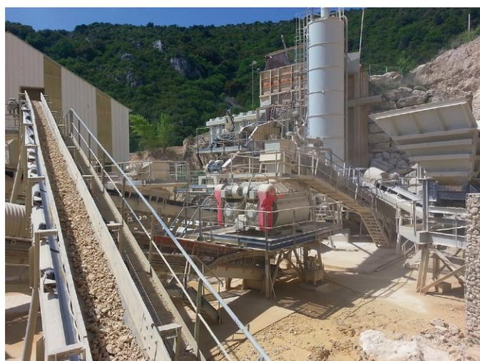
Fig. 5. The Combimix system (DKXC) in a CEMEX France processing plant for the dry treatment of clay-and-rock mixtures, located in the South of France.
