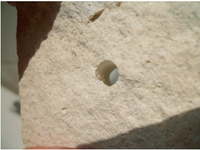
Fig. 4. Exfoliation of the hole surface under uniaxial compression of limestone specimen.
