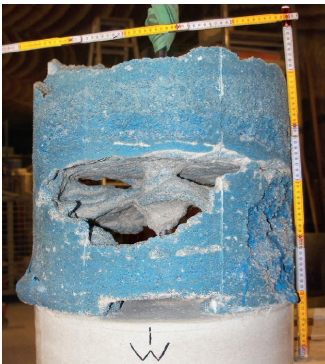
Fig. 6. Reinforced injection body as the result of a pilot-scale test to inject crushed salt (compaction density 1.52 g/cm 3 , porosity 30% by vol.) with MgO-NaWG mixtures. The non-injected areas of salt were removed by mechanical means.
