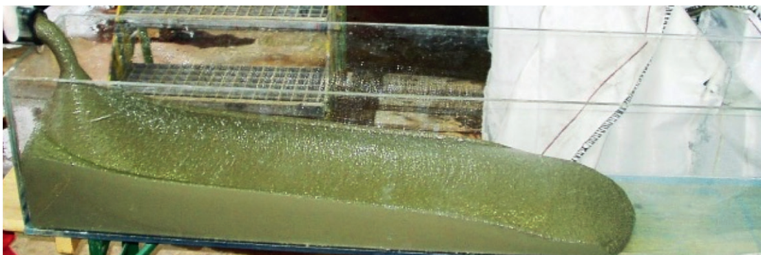
Fig. 1. Flow test with a non-sedimenting stowing material.
