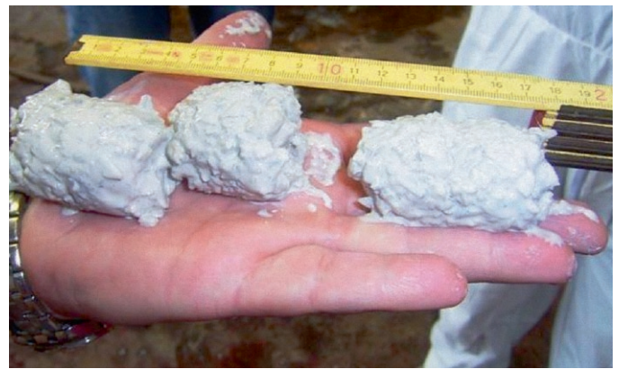
Fig. 3. Filter cake from a building material. Bild 3. Filterkuchen eines Baustoffs. Photo/Foto: DMT
