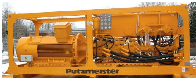
Fig. 10. Hydraulic pack, 400 kW power class.
