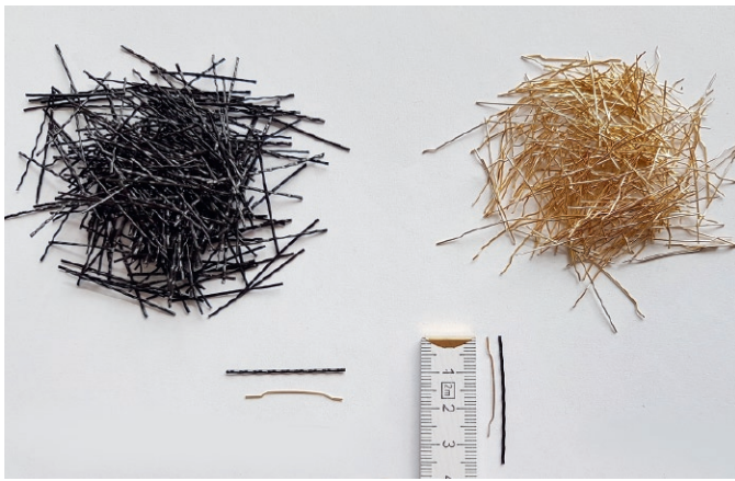
Fig. 12. Geometry of the fibres – made of polymer (left) and steel (right). Bild 12. Geometrie der Polymer- (l.) und Stahlfasern (r.). Photo/Foto: SBK
