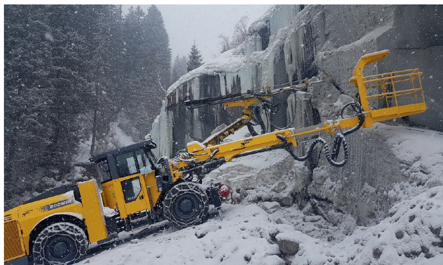
Fig. 2. Boomer E1C-DH in operation during winter time. Bild 2. Boomer E1C-DH in Betrieb im Winter. Photo/Foto: Epiroc
