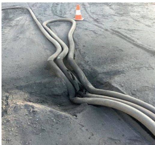
Fig. 7. Typical damage to trailing cables due to poor visibility.
