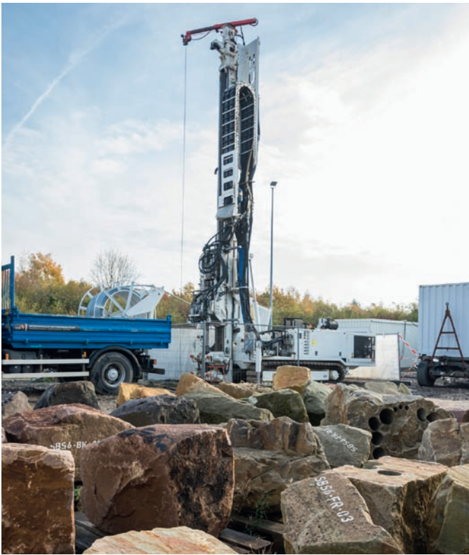
Fig. 3. BO.REX (Bochum Research and Exploration Drilling Rig) is a mobile 60 t drilling system for depths of up to 1,500 m. The Fraunhofer IEG is using it in its TRUDI demonstrator in Bochum and soon in the Rhineland demonstrator.
