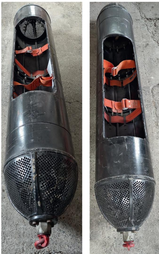
Fig. 3. Drill hole rescue cages (Dahlbusch bombs) for inclined and vertical drill holes at the BG RCI Center of Mine Rescue Services in Herne.
