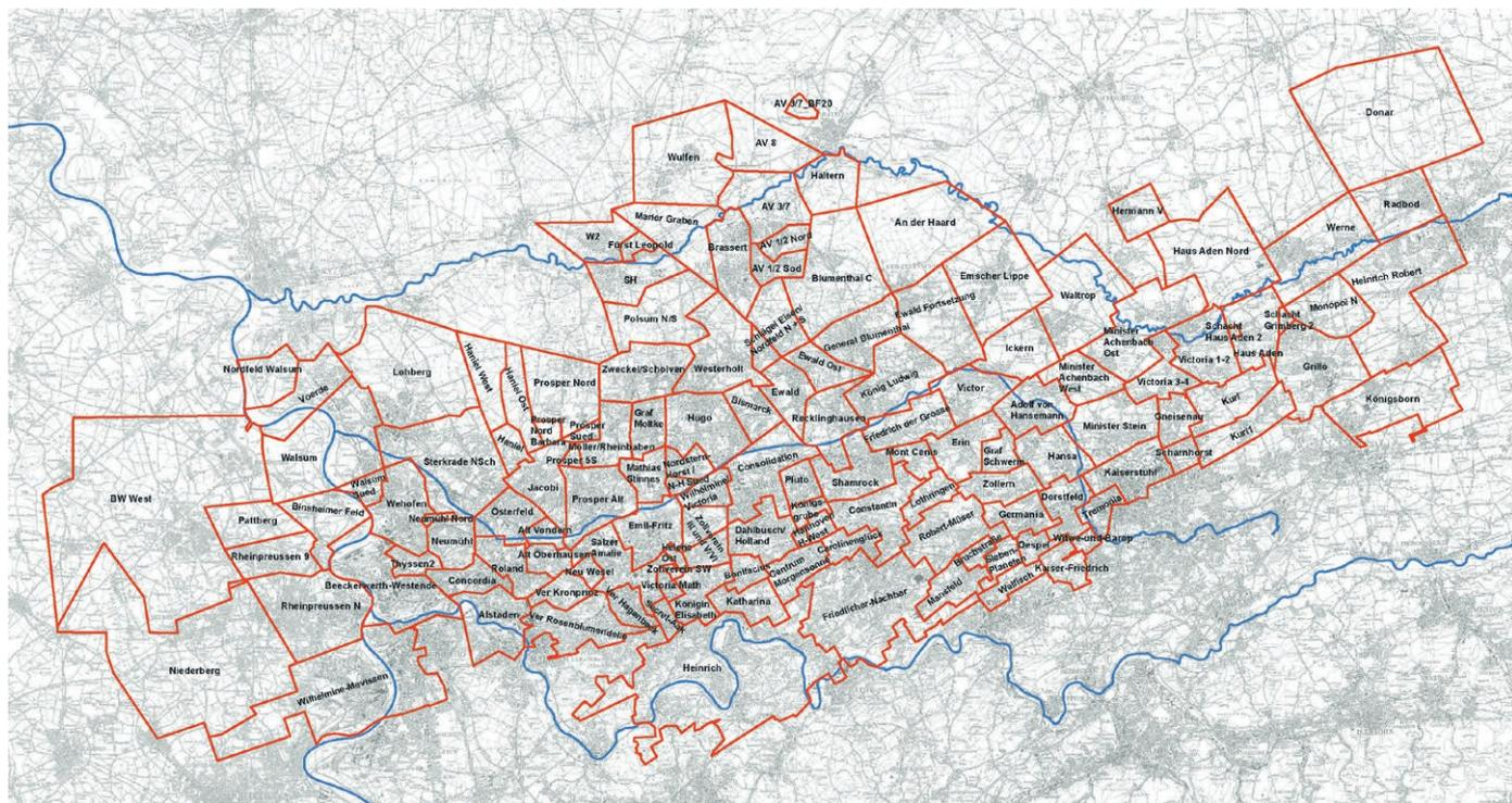
Fig. 6. Numerical mine water model Ruhr area, simulation programme Boxmodell, horizontal discretisation.
