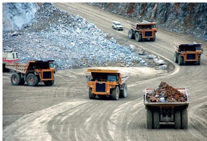
Fig. 3. Transport of extracted material via heavy-duty trucks. Bild 3. Transport des gewonnenen Materials mittels SKW. Photo/Foto: Rheinkalk GmbH
