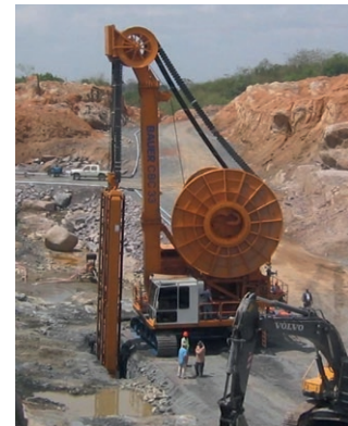
Fig. 8. Cutter mining of kimberlite veins in Sierra Leone. // Bild 8. Cutter Mining von Kimberlit-Dikes in Sierra Leone. Photo/Foto: BAUER Maschinen GmbH
