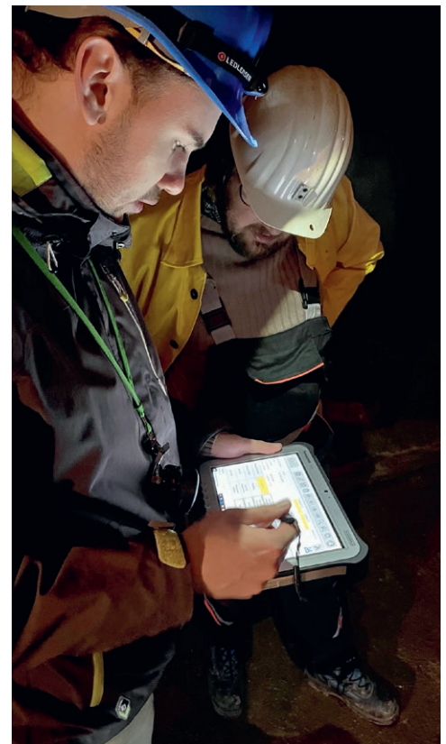
Fig. 2. advangeo® Field Cap used for capturing general outcrop data and XRF measurements in an underground mine.
