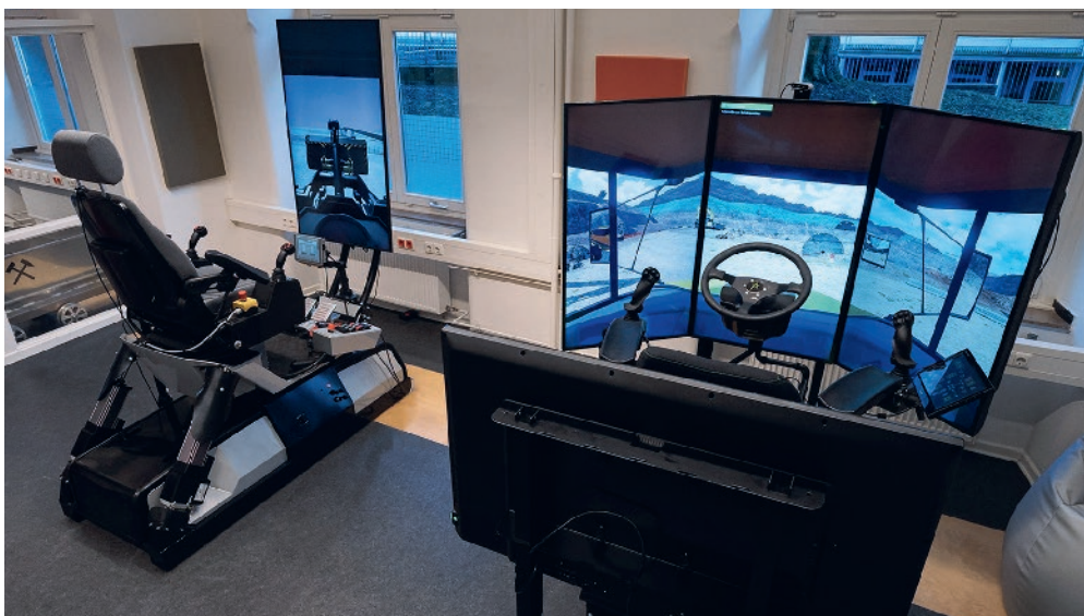
Fig. 1. Training simulators at the Institute of Mineral Resources Engineering (MRE) of RWTH Aachen University, giving students a realistic experience with virtual mining equipment.
