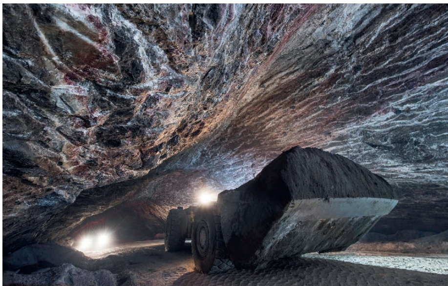
Fig. 8. LHD (LTF 10) driving a full shovel into the backfill cavity.
