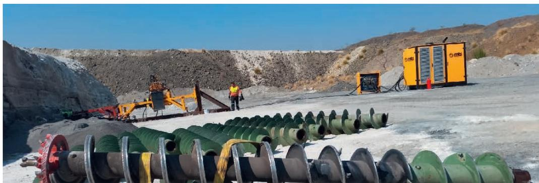
Fig. 2. Overview of test site with machine, aggregate, augers and extracted chrome ore.
