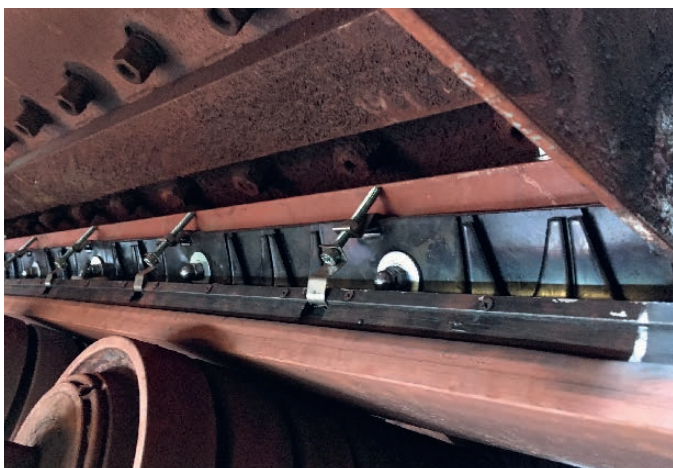
Fig. 1. With the AirScrape system, ScrapeTec has developed a concept for dedusting conveyor systems that is as simple as it is effective.
