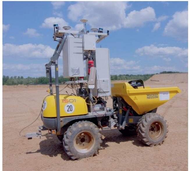
Fig. 4. Articulated dump truck with integrated M2X gateway.
