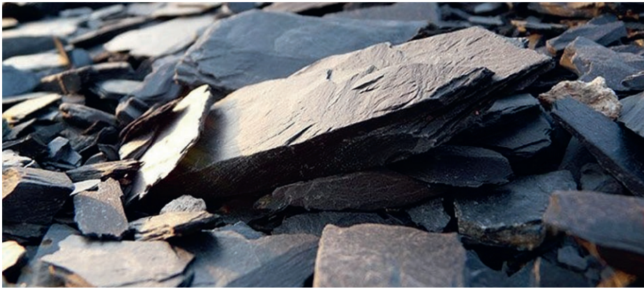
Fig. 1. Slate is composed of many overlapping and thinly-bedded layers of rock and foliated structures.
