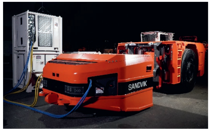
Fig. 2. Sandvik LH518B with charging infrastructure.
