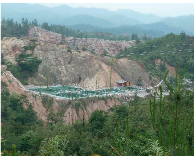
Fig. 5. Tailings ponds used in rare earth mining contain a variety of toxic chemicals and radioactive elements.
